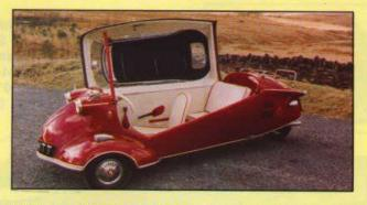
Entry is gained by raising the top lifting canopy. The drivers seat lifts back and up giving easy access. The passenger sits in tandem behind the drivers seat with legs outstretched. Sliding windows and a Cabrilot top accommodate all weather conditions.
