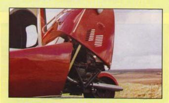
With the top lifting section open the back can be raised giving excellent access to the engine bay, where any checks and adjustments can easily be made. The main fuel tank no longer sits over the engine but is housed under the rear seat and fed via a fuel pump to a header tank over the carburettors.
