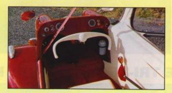
The cockpit area displays a very clear and basic instrument panel. Situated on the right is the gear lever, which is a sequential gear change. The handbrake lever is also on the right and falls easily to hand. Unique to the Schmitt is the handlebar arrangement which is used in a direct steering link giving very positive control over the car. The pedal arrangement are as normal, clutch, brake and accelerator with a floor mounted dip switch.
